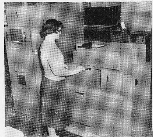
Cathie Murray operating the 604/521 Calculating Unit —the 083 Sorter can be seen in the background.
