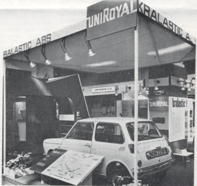
This view of the Uniroyal stand at Plastex '68 shows the rear of the Honda. The boot area is injection moulded in Kralastic and indistinguishable from the body.
